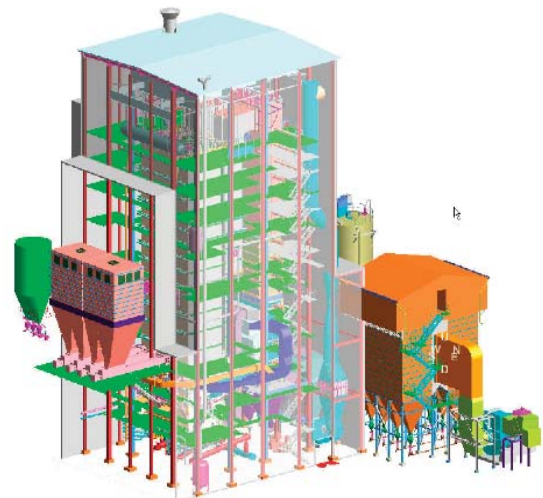
70 MWe Circulating Fluidized Bed Steam Generator for LUKOIL
