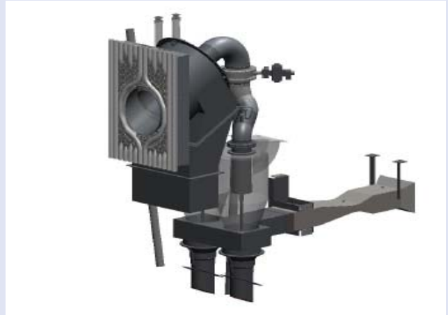
Low NOx Burner Design of Compostilla Power Plant
